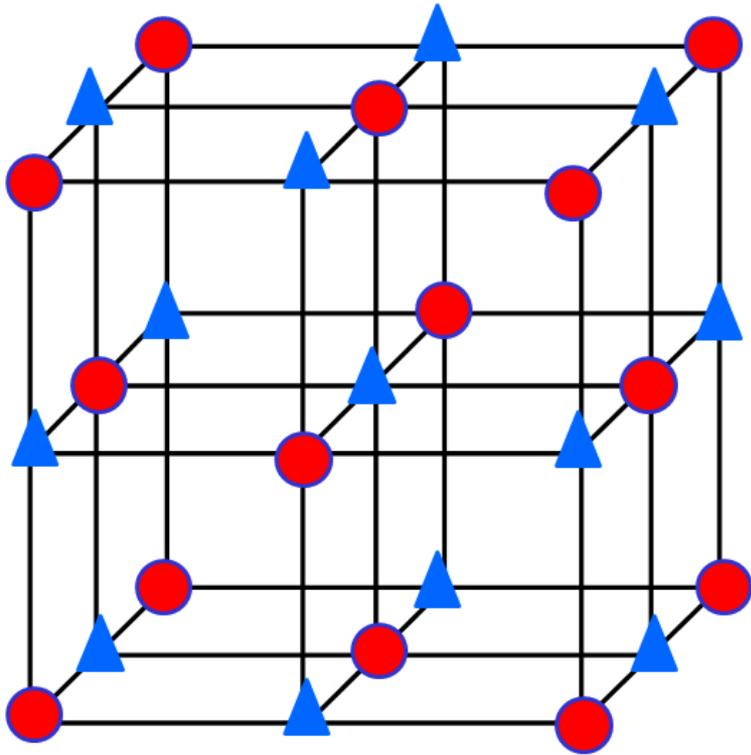
$$\text{Or } a = 2R_{\text{CFC}} + 2r_{[6]}$$
