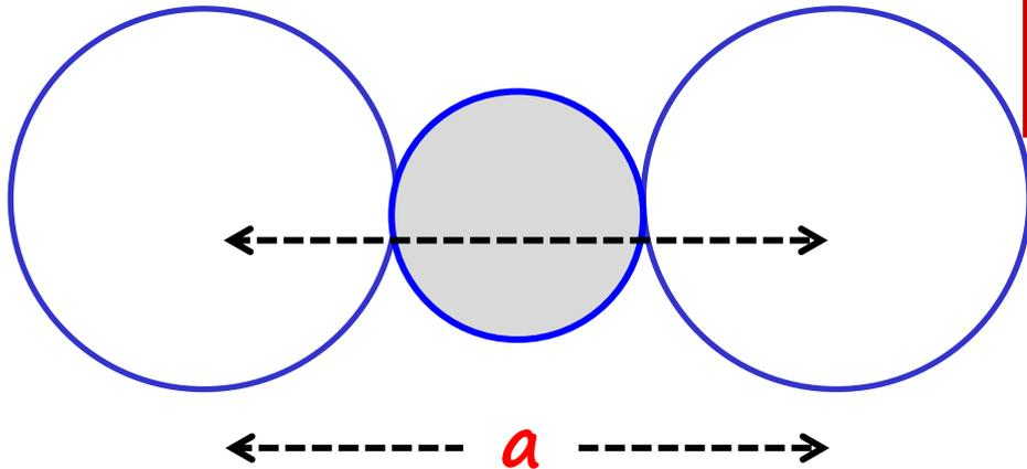
$$r_{[6]} = R_{\text{CFC}} \cdot (\sqrt{2}-1)$$
