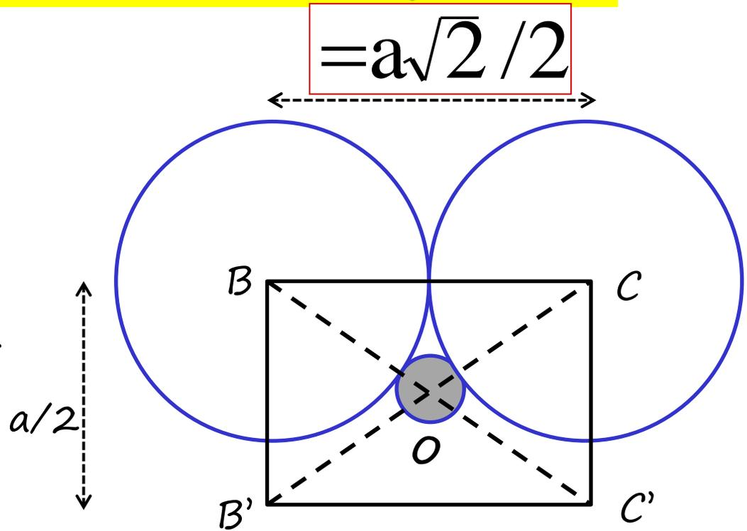
$$BC' = 2 \times BO = 2 \times (R_{CFC} + r_{[4]}) = a\sqrt{3}/2$$
